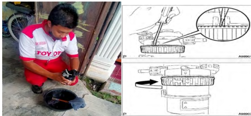
Gambar 3.28 proses membuka elemen filter
