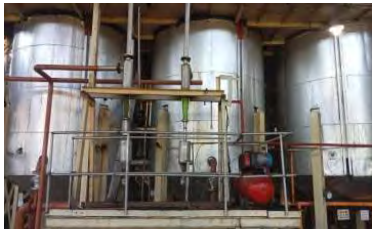
Gambar 3.19 Sand Trap Tank
