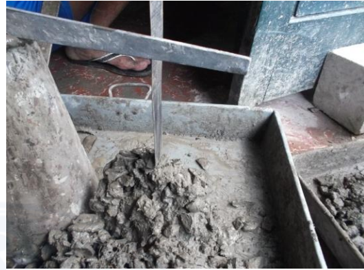
Pengukuran Slump Beton Normal
