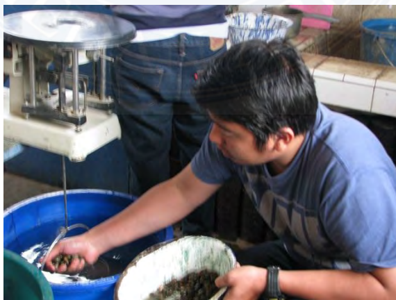
Menimbang agregat kasar didalam air
