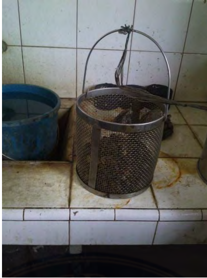
Alat penimbang agregat didalam air
