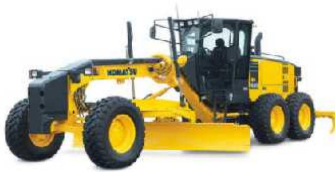
Gambar 2.7 Motor grader
