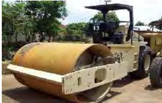
Gambar 2.10 *Vibration roller*
