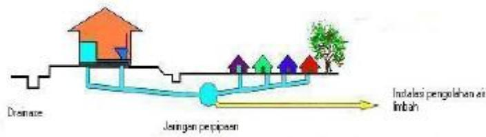
Gambar 2.8 Skema Small Bore Sewer
