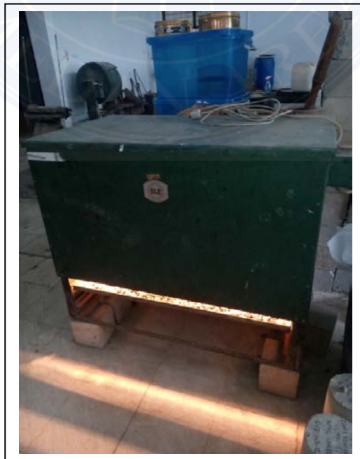
Gambar 3.8 Oven pengering agregat
