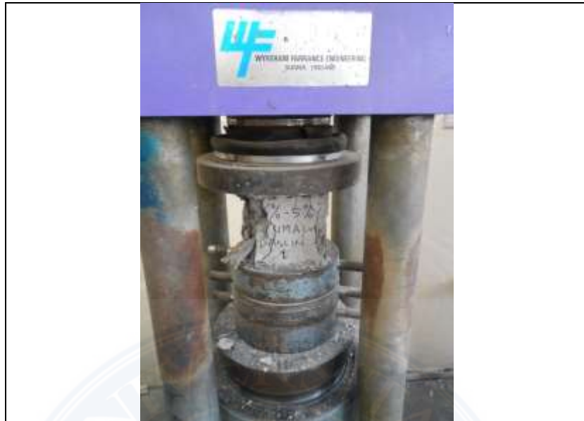
Tampak Beton pecah
