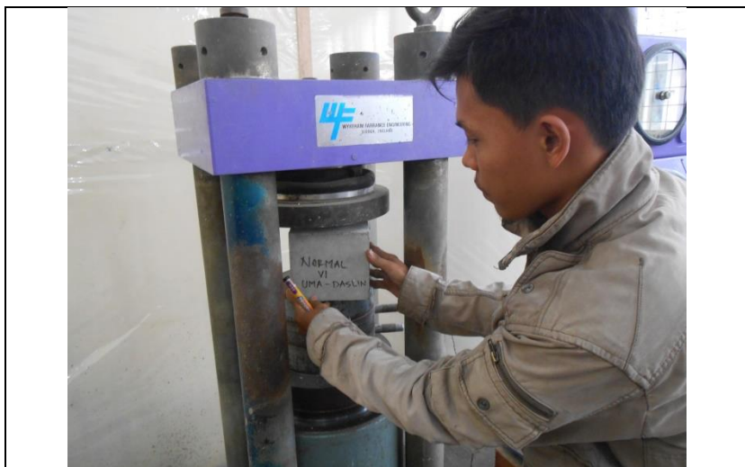
Concrete Compression Machine
