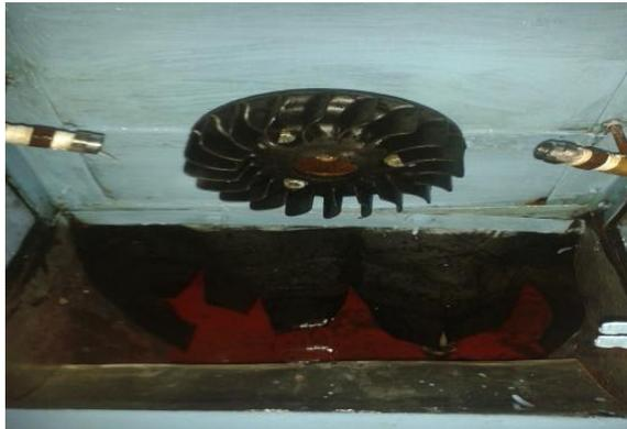
Gambar 3.17 Jarak *Nozzle* Terhadap Sudu Turbin Pelton
