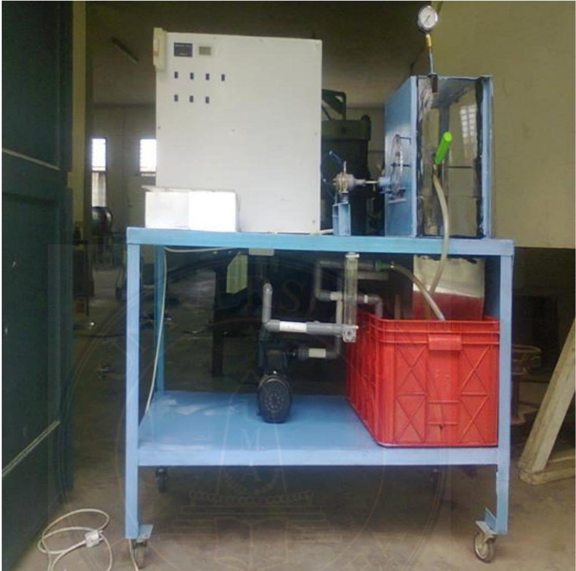
Gambar 3.0 *Design Turbin Pelton*
