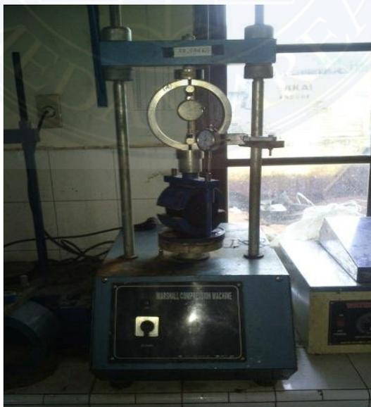
Gambar 3.2. Alat Uji Marshall
