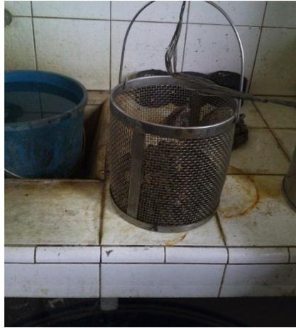
Alat penimbang agregat didalam air
