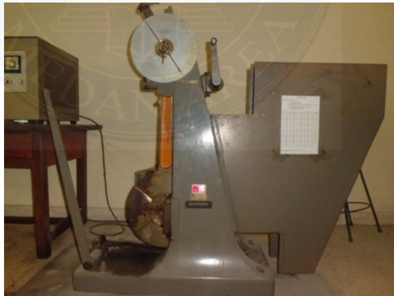
Gambar 3.3. Alat Uji Impact Metode Charphy
