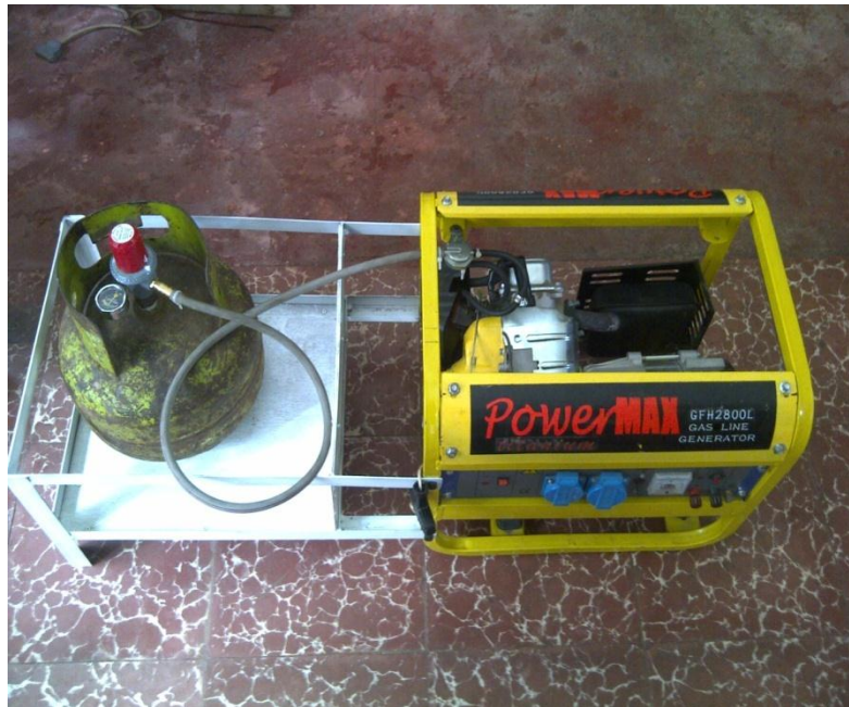
Gambar 2.2 genset bahan bakar gas LPG
