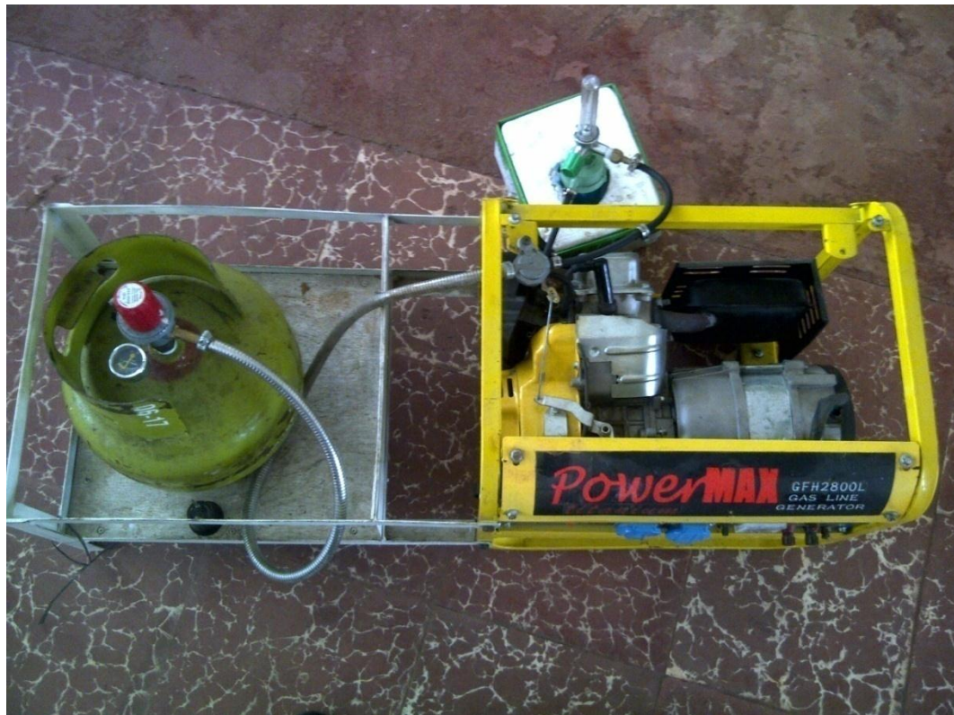
Gambar 2.22 Genset bahan bakar gas LPG
