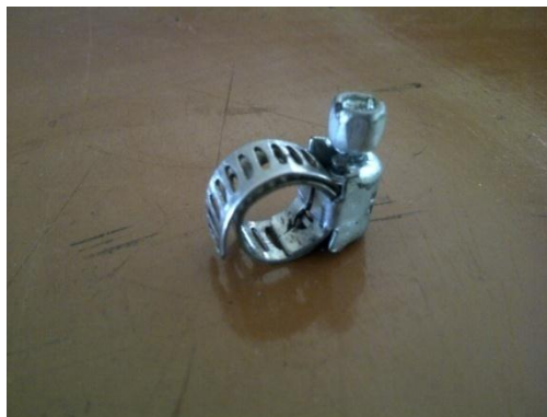
Gambar 2.12 Klem selang gas LPG
