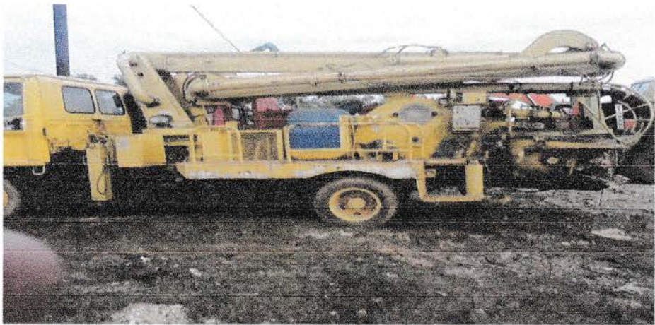
Gambar ; Pump Concrete
