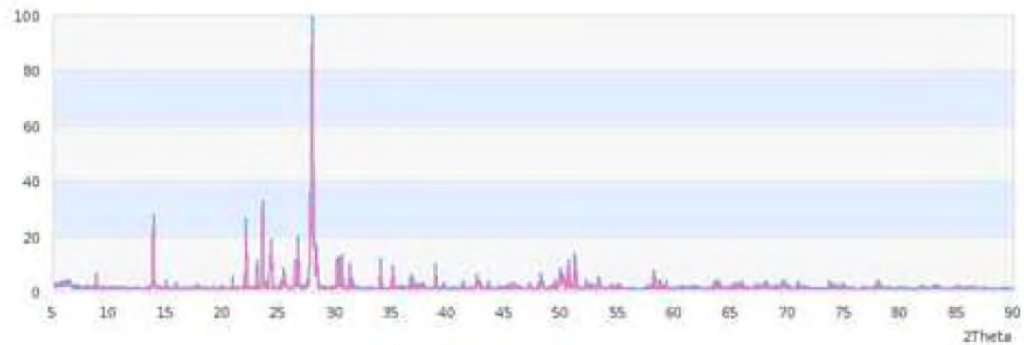
Gambar 2.2 Difraktogram Albit (Sumber: RRUFF project at University of Arizona)
