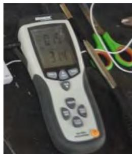
**Gambar 3.5 Hotwire Anemometer Merek Krisbow**
